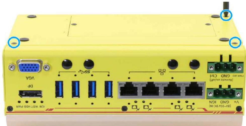
5. Remove the screw shown in the illustration and remove the CAN/ DIO panel.
