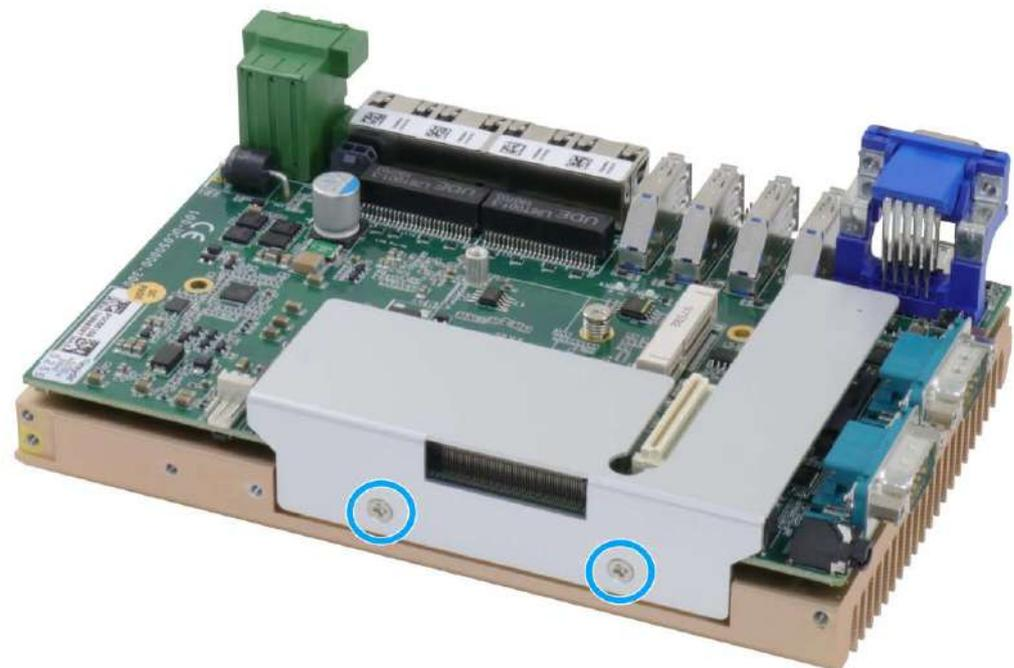
8. With external panels and DRAM/ NVMe heat spreader removed, you are ready to install internal components.
