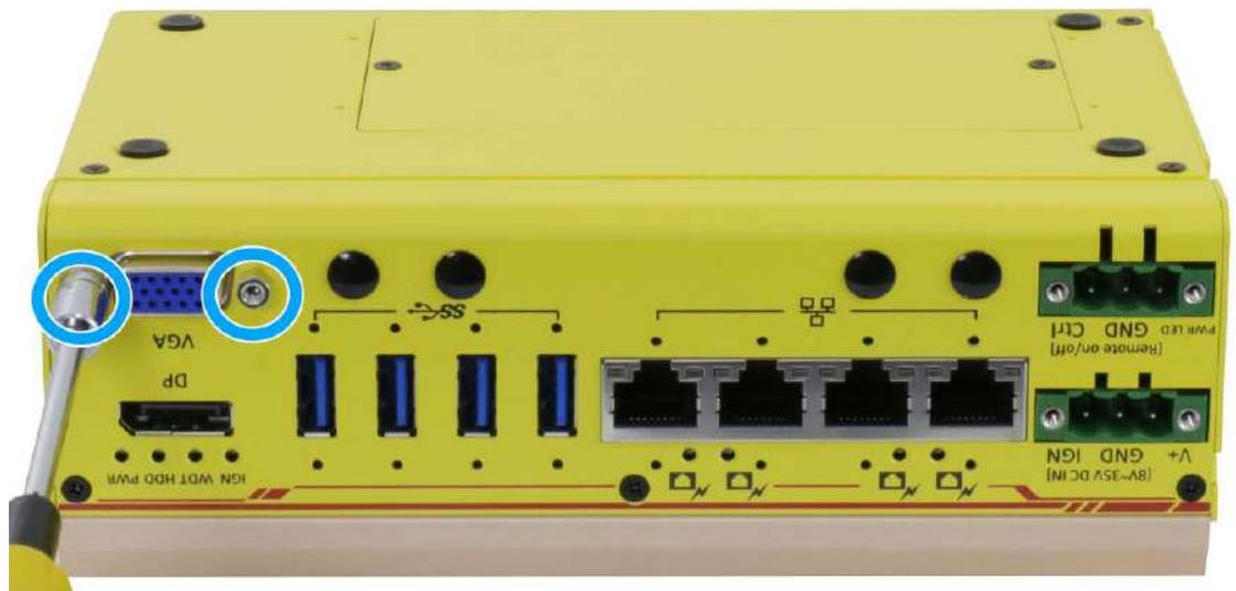
3. On the back of the system, remove the two screws indicated.
